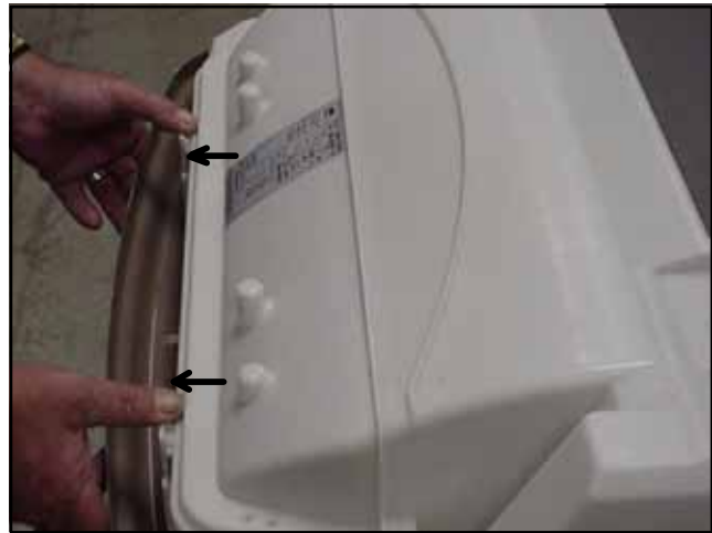
Figure 3-28 Upper Scroll Assembly Keeper Tab Release
