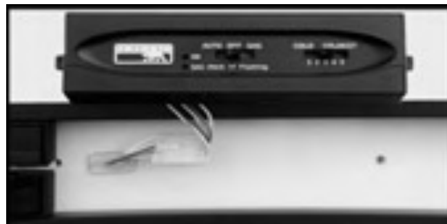
Figure 38. Wire Harness Connection.
