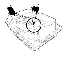
per. If you are using the weld on the process valve, be sure the valve core is removed before any heat is applied.
