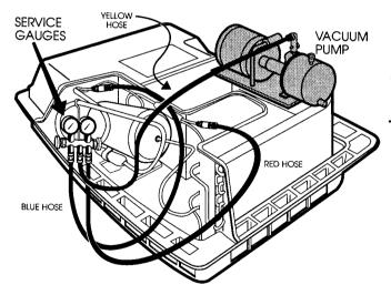
Check all hose connections for tightness. If the low side gauge does not change, there is a leak in the sealed system. Locate the leak and correct it before proceeding.
