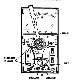
If nothing operates on the air conditioner, remove the return air grille assembly and verify the red, orange, yellow and blue wires are properly connected (red to red, orange to orange, etc.). Next disconnect the red wires and check for 12 volt D.C. between red wire from roof section and the orange or blue wire from roof section. If no voltage is received, refer to section 4.5. If voltage is received, the problem lies with the thermostat or thermostat wires.
