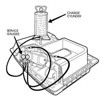
Now the blue low side and the red high side lines should be disconnected. Make sure that the air conditioner connection is sealed before removing the lines. The process tube can be pinched off in two places; the charging port cut off, and the end of the tube brazed for a hermetically sealed system.
