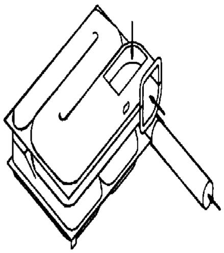
TO CLEAN THE CHAMBER, THE FURNACE MUST BE REMOVED FROM THE CABINET AND THE MANIFOLD BLOWER ASSEMBLY, AND THE CONTROLS REMOVED LEAVING THE CHAMBER ONLY. AS SHOWN. USING COMPRESSED AIR, BLOW THROUGH THE CHAMBER, AS SHOWN BT ARROWS TO REMOVE SOOT OR LOOSE DEBRIS.
