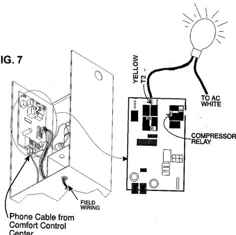
Use an AC light bulb to test if the relays on the board are completing a circuit. Check from the common (white wire) to:
