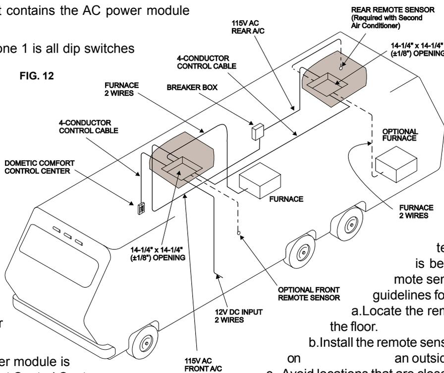
If a furnace is operated by the Comfort Control Center, the thermostat wires are attached to the two (2) blue wires from the control box. The furnace dip switch for that zone (control box or power module) is turned on.
