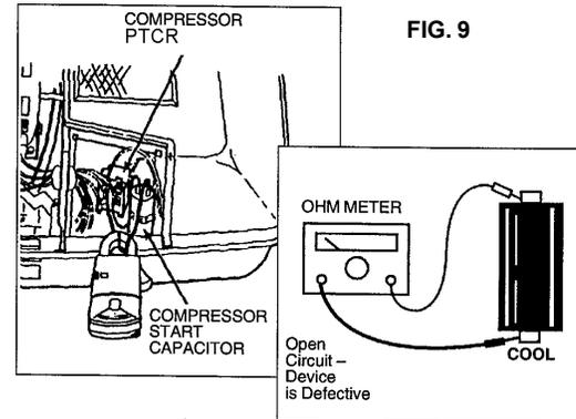
2. The second check is an amp reading. Clamp an ammeter around the wire from the start capacitor. See FIG. 9. Turn on the AC power and set the Comfort Control Center to the cooling mode. When the compressor starts, the ammeter should show a reading for approximately one second. If there is no amperage reading or a prolonged reading, the PTCR is faulty and must be replaced.
