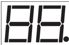
If the screen segments do not match the ones shown in the illustration, the fault is in the optical control assembly. Replacing the optical control should resolve the fault.
