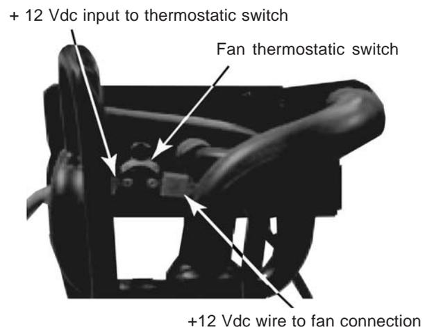
Figure 25. Fan Thermostat.
