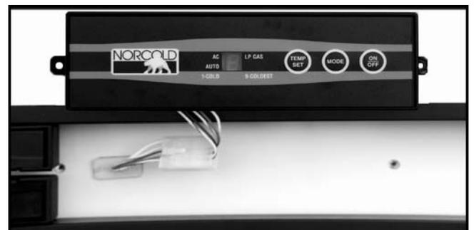
Figure 41. Wire Harness Connection.
