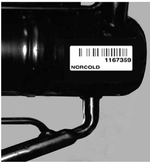
Figure 2. Cooling Unit Bar Code Label Location.
