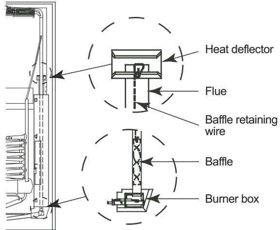
Figure 14. Flue and Components.
