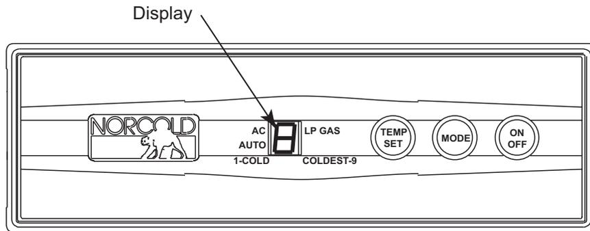
Figure 45. N62X0/N82X Optical Control Assembly.
