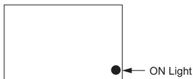
The ON light should be the only LED displayed. If any other LED displays, the fault is in the optical control assembly. Replacing the optical control should resolve the fault.
