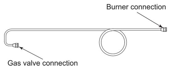
Figure 13. Burner tube.
