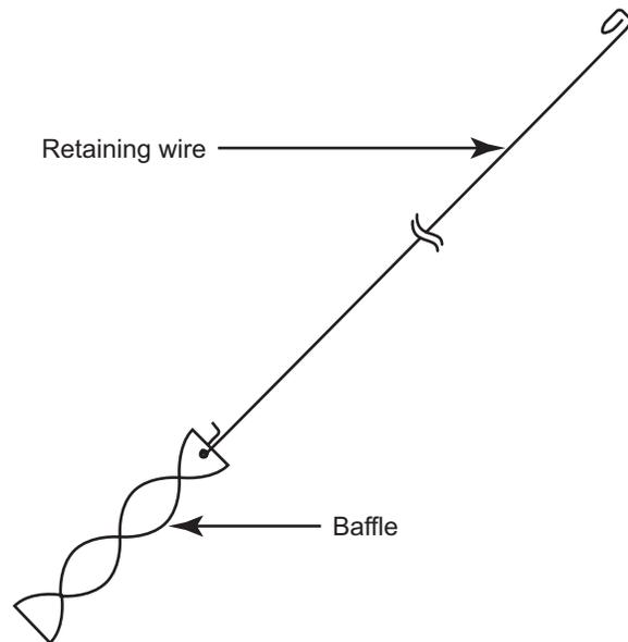
Figure 15. Flue Baffle.
