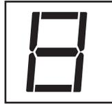
If the LED segments do not match the illustration, the fault is in the optical control display.
