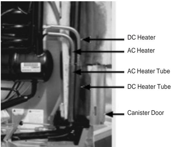
**Figure 20. AC and DC Heaters (3-way refrigerator)**
