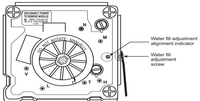
Figure 53. Water Fill Adjustment Screw and Indicator.
