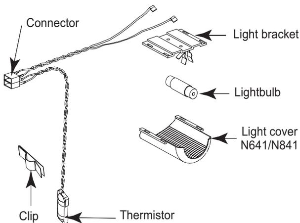
**Figure 21. Lamp/Thermistor Assembly.**
