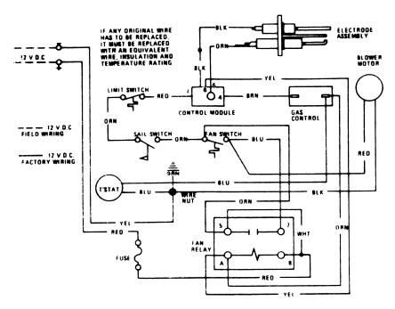
Preliminary checks: (1) Input polarity. If a spark is present and the gas valve opens for the flame establishing period but then locks out at the end of three to ten seconds, check the input voltage at Terminals 1 and 6 for the proper polarity. Terminal 1 should be "hot"; 12VDC (05-15) with respect to ground. Terminal 6 is neutral, or zero voltage, with respect to ground. (See Figure 1).
