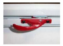
Each exit latch is attached to the window frame using two small screws and nuts. Remove these with a Phillips head screwdriver and a small wrench. Discard the defective latch. Some windows include a metal stiffener bracket on the back of the latch and frame. These must be reused with the new latches. Place the new latch into position and align the holes of the latch, frame and stiffener. Secure the new latch with the screws provided. Check for ease of opening and secure closure.
