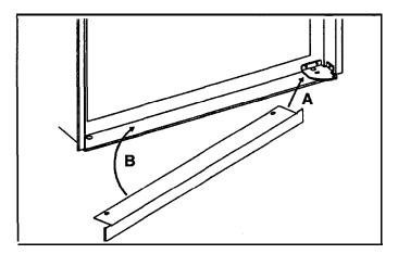
C. When the front strip is in place, install one screw through the hinge and into the floor. The second screw is installed with a washer on the opposite side.
