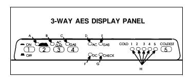
The AES mode of operation takes priority over all other operating modes. If more than one mode selector button (2), (3) or (4) is in the down position, the priority is from left to right.
