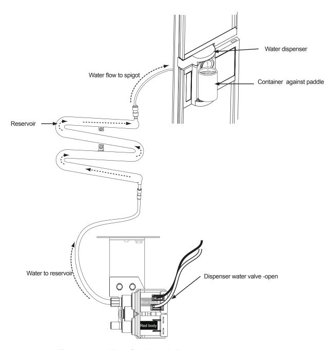
Figure. 10-4. — Water flow through dispenser system.
