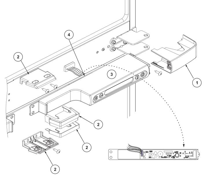
Figure 6-10. —Control panel and related components.
