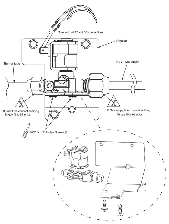
Figure 4-3. —Gas valve replacement.
