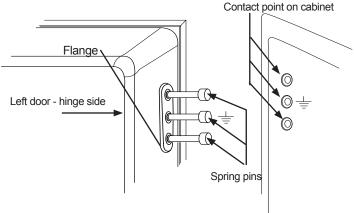
Figure 5-10. —Spring pins and cabinet contacts.
