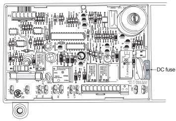
Figure 5-2. —DC power fuse location.
