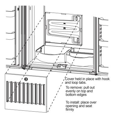
Figure. 10-8. —Cover for reservoir recess.
