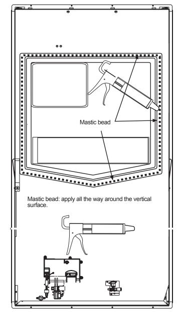
Figure 7-8. —Mastic application on cabinet opening.
