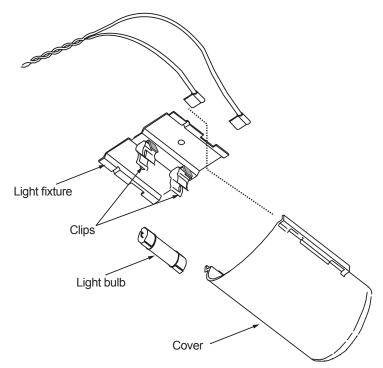
Figure 5-4. —Light fixture assembly.
