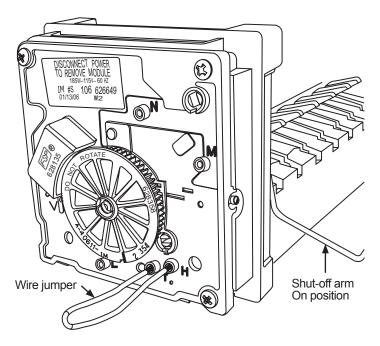
Figure 9-9. —Cycling the ice maker manually.
