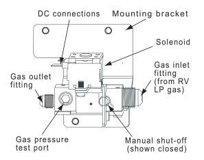
Figure 9. New Style Solenoid Gas Valve.
