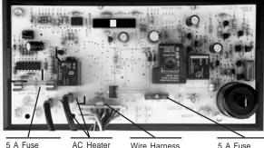
5 A Fuse AC Power (F3) AC Heater Wire Harness Terminals Connector (P1) 5 A Fuse DC Power (F1)
