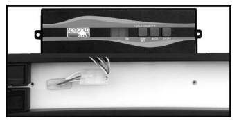
Figure 44. Wire Harness Connection.
