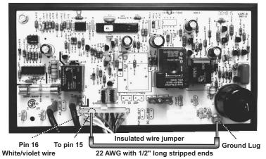
Figure C. Resetting Power Board.
