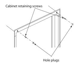
Figure 32. Top retaining screws and hole plugs.
