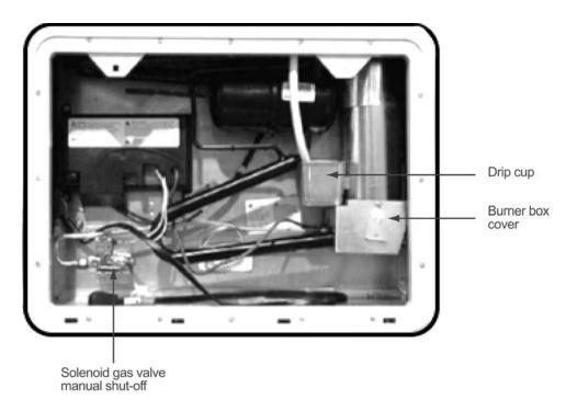
Figure 17. Drip Cup and Burner Box Cover.
