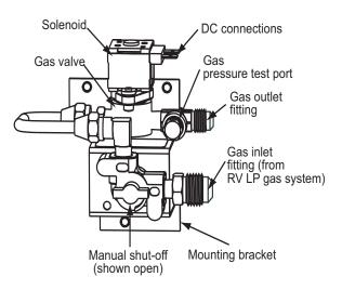
Figure 10. Old Style Solenoid Gas Valve.
