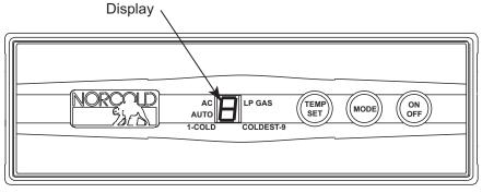
Figure 45. N62X0/N82X Optical Control Assembly.
