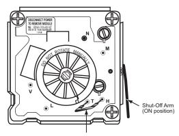
Insulated Jumper Wire (14 AWG with 1/2" stripped ends)
