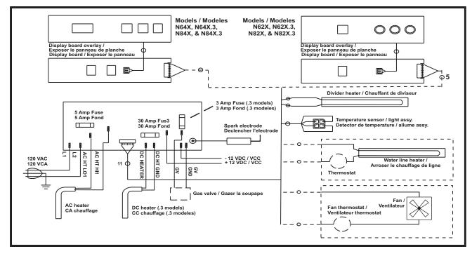
N62X/N82X/N64X/N84X/N64X.3/N84X.3 Wiring Pictorial – Units with serial number 851759 and higher.
