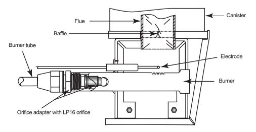
Figure 18. Burner and Components.
