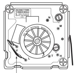
Insulated jumper wire (14 AWG with 1/2-stripped ends)
