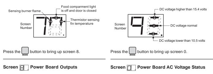
Screen 8 displays "live" power board outputs using Screen 0 displays AC voltage status using lighted LED lighted LED segments. The illustration below provides segments. The illustration below provides AC voltage "live" outputs information and assigned LED segments. status information and assigned LED segments. If AC If a power board output is active or "live," its voltage at the power board within normal range (108 assigned output LED will be on. to 132 Vac), LED segment 4 will be on.
