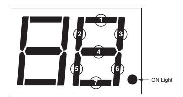
Figure 48. Diagnostic LEDs Segments Identification.
