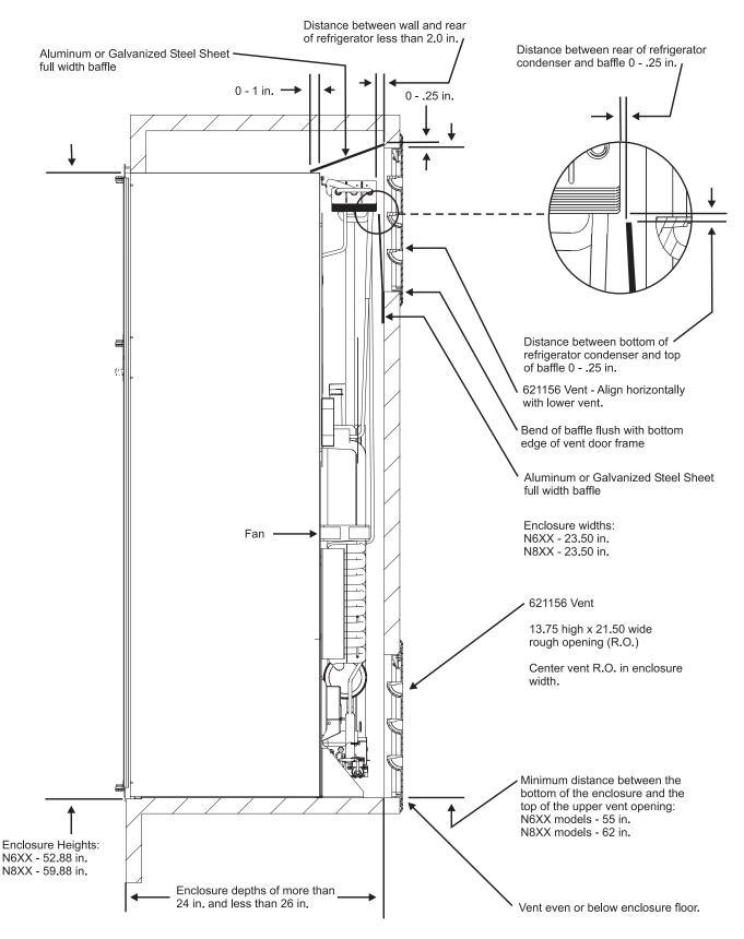
Figure 6. Baffle Arrangement for Enclosures Depths of More than 24 Inches and Less than 26 Inches.
