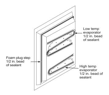
Figure 30. Application of Sealant.
