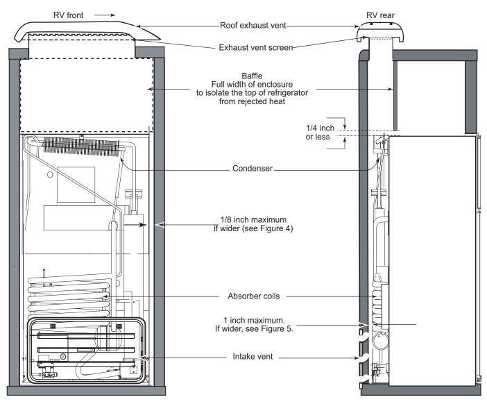
Figure 3. Roof Exhaust Venting Arrangement.
