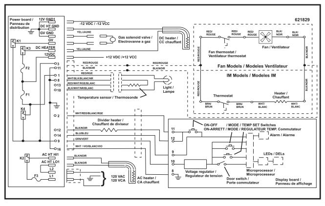
N62X/N82X/N64X/N84X/N64X.3/N84X.3 Wiring Schematic – Units with serial number 851759 and higher.
