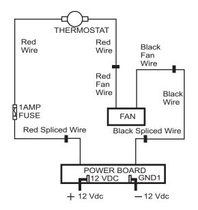
Figure 27. NORCOLD Fan Kit Wiring Pictorial.
