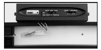
Figure 38. Wire Harness Connection.
