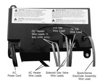
Figure 34. Power Board, 3-Way with Cover
