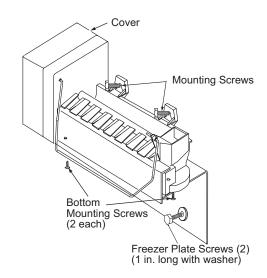
Figure 50. Ice Maker Mounting Hardware.
