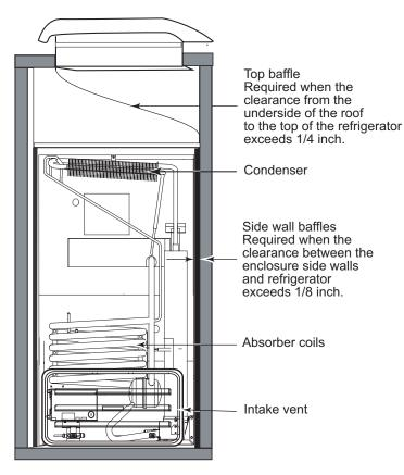
Figure 4. Rear View–Roof Exhaust Venting.
