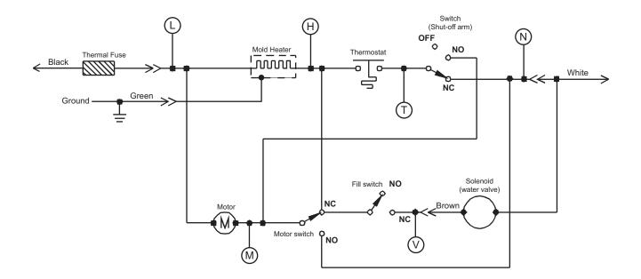
N64X IM/N84XIM – Wiring Schematic for Ice Maker Wired to Refrigerator AC Cord.
