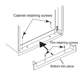
Figure 31. Bottom trim and retaining screws.
