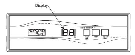
Figure 47. Models N64X/N84X Optical Control Assembly.
