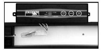
Figure 41. Wire Harness Connection.
