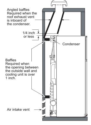
Figure 5. Baffles Required for an Inboard Roof Exhaust Vent Installation.
