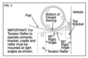
F. Carefully climb ladder. With tension rafter still resting on the ground, position the top bracket/pad assembly against the vehicle so that the top cradle of the tension rafter touches the bottom of the closed awning as shown in FIG. 3.
