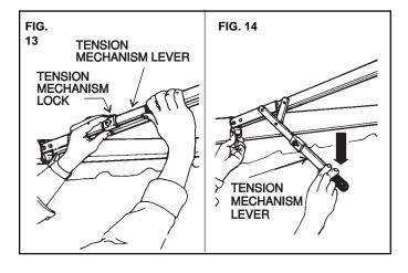
15. Loosen adjustment knob on side of tension rafter and push tension mechanism lever up. Slide tension mechanism lock down. (FIGS. 14A, 14B & 14C)
