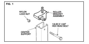
NOTE: If the Optima Center Support is being used in conjunction with the Optima Tension Rafter, the roller bracket is not required and the center support should be attached to the tension rafter as pictured in FIG. 2. To attach center support, use 1/4-20 nut and 1/4-20 x 2-1/2" hex head bolt in the tension rafter. Install the center support with the two rubber sleeves (provided) on both sides of the center support. (FIG. 2)
