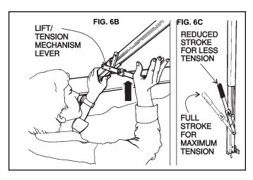
This step pushes the roller tube out and stretches the fabric taut. The tension rafter is designed to use the full stroke of the tension mechanism for 25 foot awnings. Shorter awnings may require less tension.
