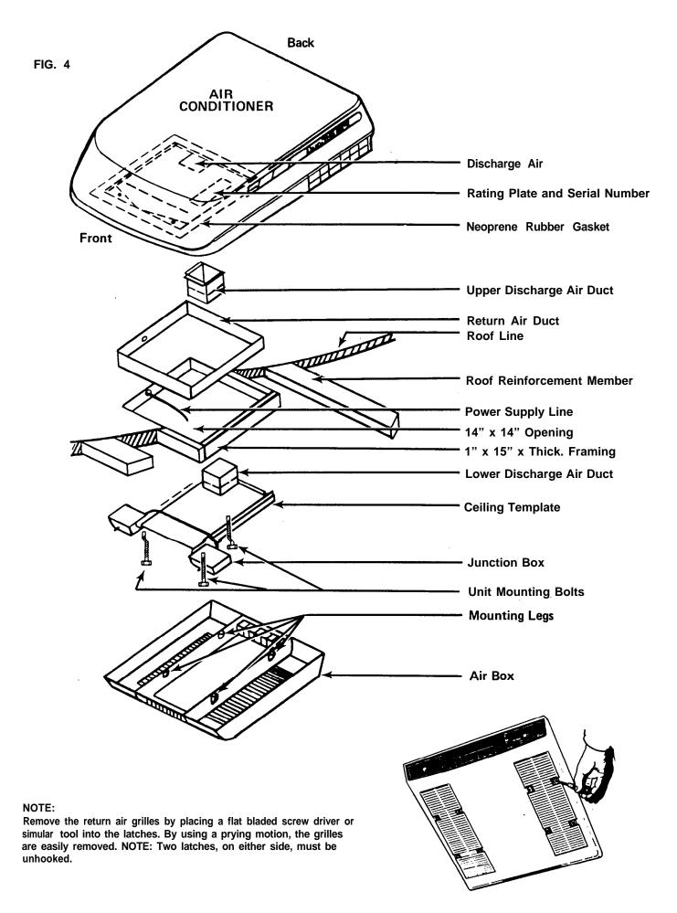
E. Evenly tighten the three mounting bolts to secure the air conditioner to the roof. The mounting bolts should be tightened to a torque of 40 to 50 in. lbs. to insure adequate air conditioner to roof seal.
