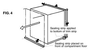
**NOTE:** Be careful not to damage the sealing strip applied to the floor of the enclosure when the refrigerator is put in place. The refrigerator is secured in the enclosure with six screws and they must be installed in the following order:
