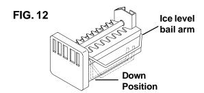
When the ice maker thermostat senses the preset temperature for ejection of the ice cubes, the fingers will start to rotate dumping any ice cubes and filling the mold with water.
