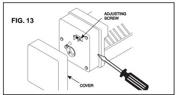
**CAUTION: DO NOT** turn the screw more than one turn at a time. The ice maker should be allowed to cycle several times before another adjustment is made. Be sure to replace protective cover on the cycle after adjustments have been made.
