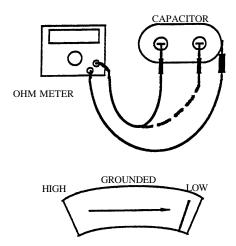
Indicator moves to the right side of the scale and stays there (indicating a completed circuit). The capacitor is grounded.
