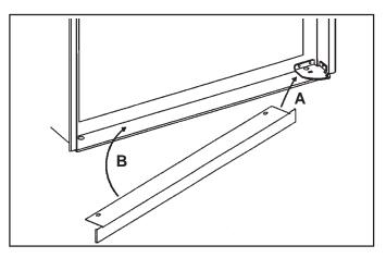
C. When the front strip is in place, install one screw through the hinge and into the floor. The second screw is installed with a washer on the opposite side.
