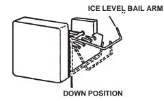
When the ice maker thermostat senses the preset temperature for ejection of the ice cubes, the fingers will start to rotate - dumping any ice cubes and filling the mold with water.
