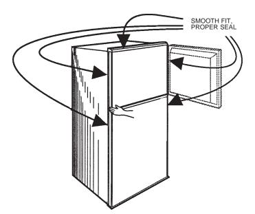
To adjust either door, loosen the hinge bracket screws, reposition the door then tighten the hinge bracket screws. To adjust up or down, add or remove washers from the lower hinge pin.
