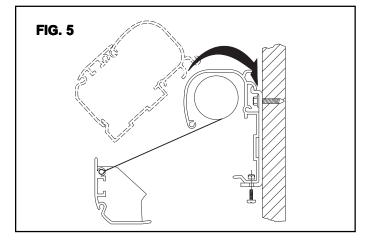
5. Using a 3/16" drill bit (7/32" bit if drilling into steel) and using the 1/4" holes drilled in Steps 2 and 3 above as guides, drill into the sidewall of vehicle. Install #14x1-1/2" screws and tighten.
