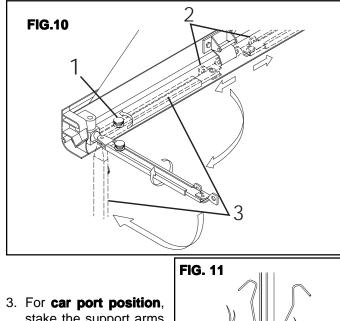
stake the support arms to the ground with stakes provided. (FIG. 11) For patio position, engage the support arm foot into the bottom mounting bracket. (FIG. 12)
