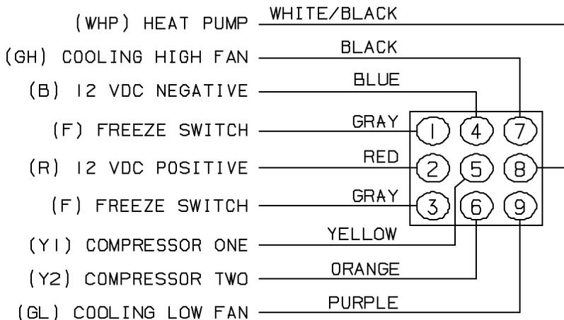
The thermostat operation switches the 12VDC + to all output terminals.
