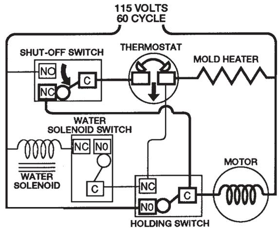
When the ejector blades reach the ice in the mold, the motor will stall. It will remain in this position until the ice has thawed loose. During this time the mold heater remains energized.
