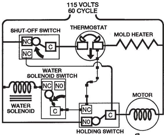
Near the completion of the first revolution, the timing cam closes the water valve switch. However since the thermostat is still closed the mold heater circuit is energized. Current will not pass through the water valve solenoid and its switch. (Electrical current follows the path of least resistance.)
