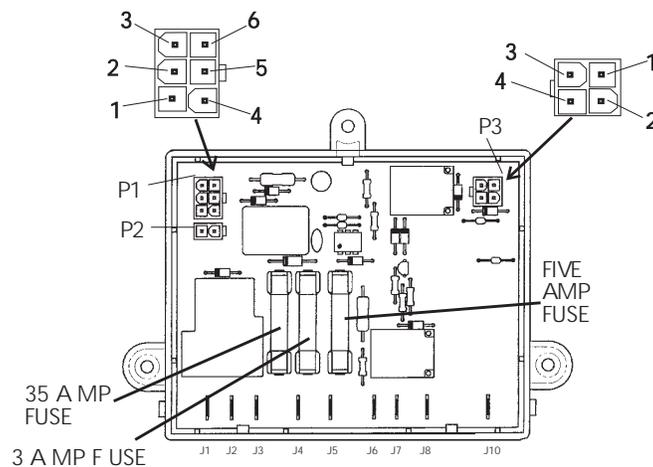
**B. AC MODE:** Check that incoming AC voltage is present at terminals J5 and J6 on the circuit board. Check for voltage at the heating element connection terminals J7 and J8 on the circuit board. If no voltage is present, check the 5-amp AC and 3-amp DC fuses. If fuses are good, replace the circuit board.
