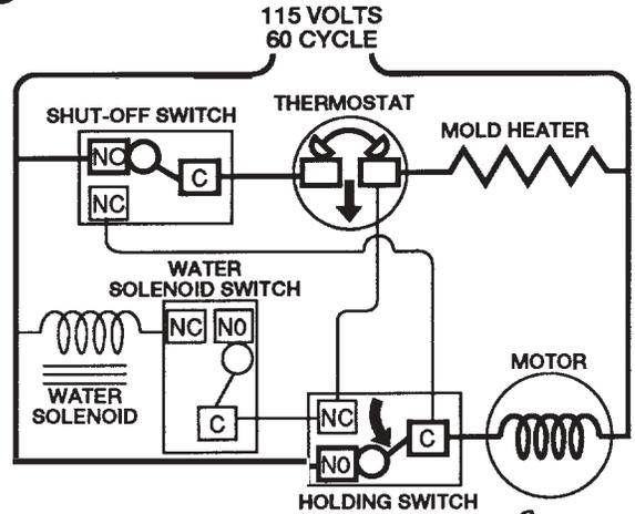
After a few degrees of motor rotation, the timing cam switches the holding switch to its normally open position; this assures completion of the cycle. The mold heater remains energized through the thermostat circuit. During the first half of the cycle, the shut-off arm is raised and lowered by the timing cam and operates the shut-off switch.
