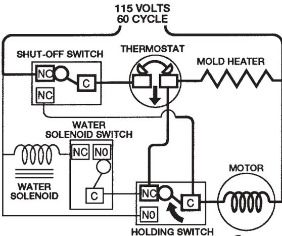
At the end of the first revolution the timing cam opens the holding switch. However, since the thermostat is still closed a second revolution begins.
