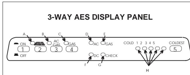
The AES mode of operation takes priority over all other operating modes. If more than one mode selector button (2), (3) or (4) is in the down position, the priority is from left to right.
