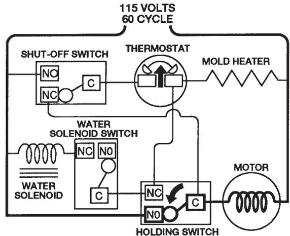
Some time during the second revolution the mold heater resets the thermostat. At this time, the mold heater is de-energized. If the storage bin is full, the shut-off arm will remain in a raised position.
