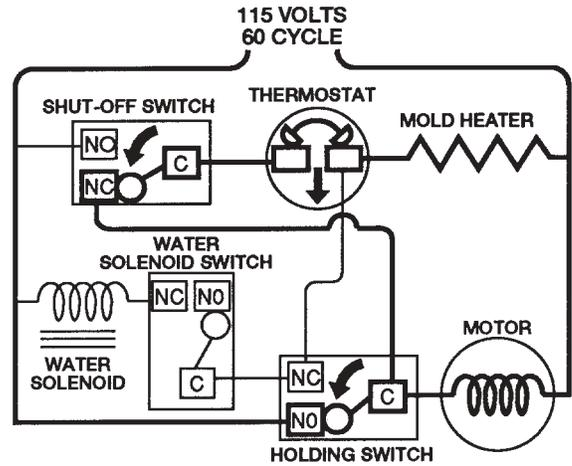
Once again after a few degrees of rotation the timing cam closes the holding switch providing a circuit to the motor that will assure completion of this revolution. The mold heater remains energized. The shut-off arm will raise and lower again operating its switch. The ice that was ejected during the first revolution is dumped into the storage bin.
