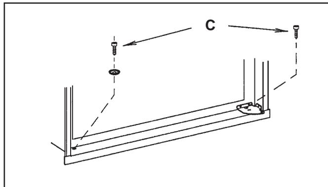
**Second: Install the two screws in the top frame.**
